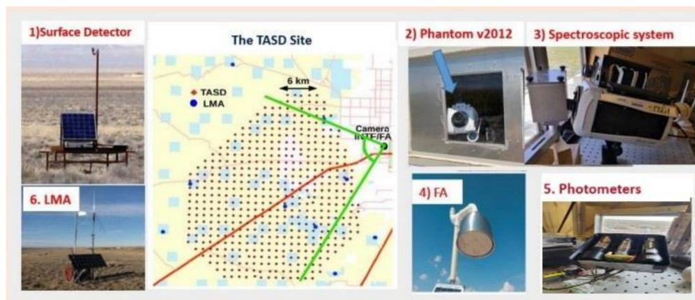
**Figure 1:** The Telescope Array Surface Detector together with the suit of lightning instruments installed at the TA site including the spectroscopic system and photometer array from which the data discussed in this work is collected.
