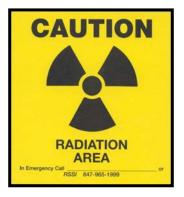
All radioactive materials and radiation-producing devices are labeled with this universal symbol for radiation. Additionally, the doors to rooms that use radioactive materials and equipment that may contain radioactive materials (for example refrigerators, equipment, radioactive waste containers, etc.) will bear the "CAUTION RADIOACTIVE MATERIALS" sign and may state "AUTHORIZED PERSONNEL ONLY". This training authorizes you to enter these areas for cleaning, maintenance, and security.
